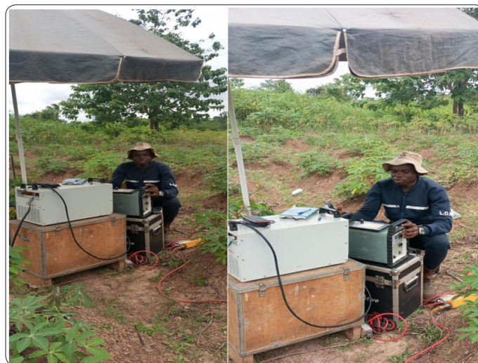
Figure 7: 2D IP/Resistivity Data Acquisition in Progress after equipment set up.
